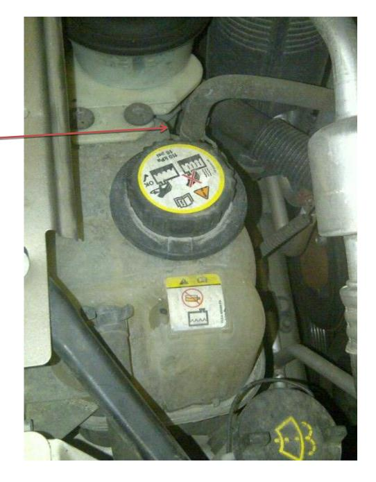
Insert Fitting A into hose Insert Fitting B onto bottle
